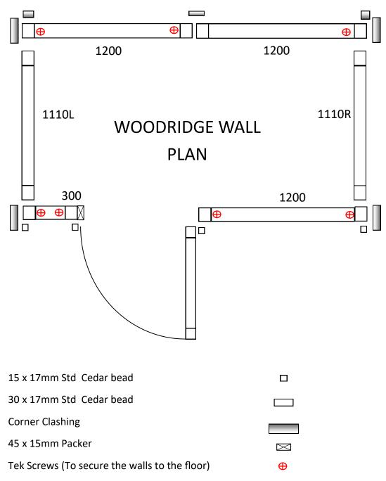
Please note: The walls are not screwed down to the floor until all the walls are erected, the roof is in place and the doors are about to be installed.
