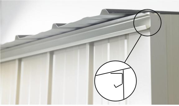
**Step 1:** Position Door Track (107) on front wall up against underside of Roof, with right hand end flush with the right hand corner. Pre-drill hole in centre and rivet in place. Remove ALL drill filings
