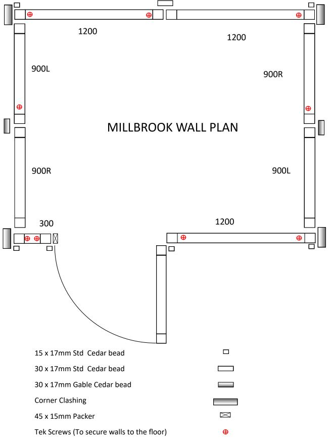
Please note: The walls are not screwed down to the floor until all the walls are erected, the roof is in place and the doors are about to be installed.
