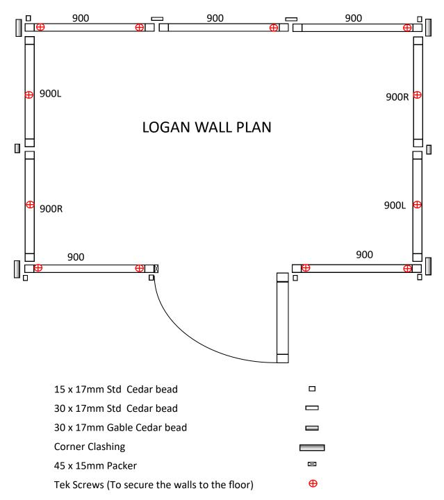
Please note: The walls are not screwed down to the floor until all the walls are erected, the roof is in place and the doors are about to be installed.
