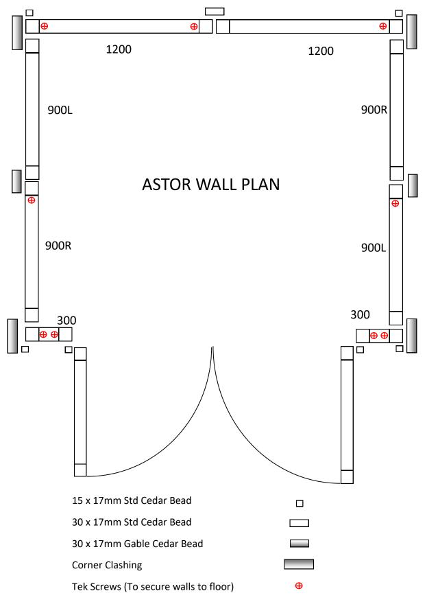
Please note: The walls are not screwed down to the floor until all the walls are erected, the roof is in place and the doors are about to be installed.
